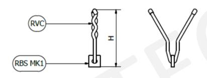
ASSEMBLED MARK 1 ROTALOCK ANCHOR SYSTEM
